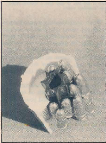
A cutaway view of the helical feed, double stacked magazine design.
